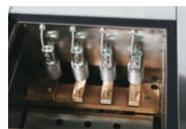
Detail: four load cells 500 N
