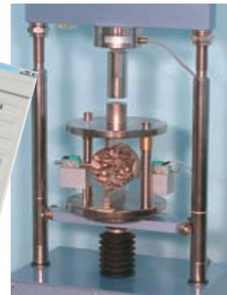
B043-02 Software splitting tensile test
